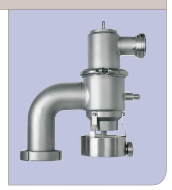
The vacuum valve housing can be cleaned during tank CIP cycle by connecting the CIP nozzle to main CIP supply. When the tank is cleaned pressureless, a small volume of cleaning fluid will pass the vacuum valve body and clean the seat. To ensure thorough flushing of valve seat, force opening of the valve is necessary - this is also done when the tank is pressureless. The use of a drain collector is recommended to prevent detergent from running over tank top.
